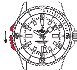
Setting 2 : bezel unlocked
