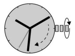
Gently turn the crown clockwise (or away from you) until you set the correct time, with the minute hand 1 minute ahead of the correct time.
