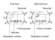
3. Press (A) to reset the stopwatch to all zeros.
