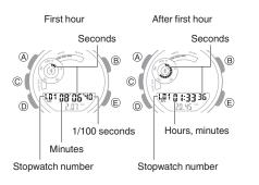
4. Press (A) to reset the stopwatch to all zeros.
